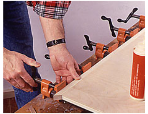
10--Begin the desktop by cutting panel to size and cutting solid wood banding to fit the edges. Miter corners of banding.
