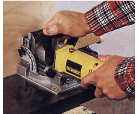
4--Cut the plate slots in the case bottom by clamping the panel to your table-saw fence and sliding the plate joiner across the table.
