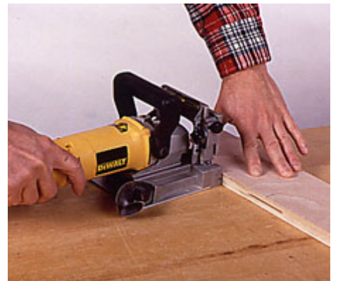
3--After cutting all the case parts to size and applying the edge tape, begin assembly by cutting plate slots in the back rails.
