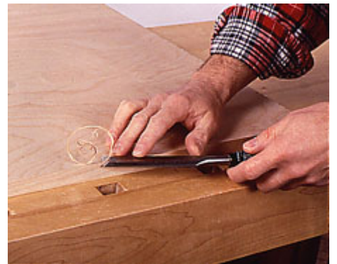
2--Trim the edging tape flush to the panel with a sharp chisel. Cut with the grain direction, not against it, to prevent splitting.
