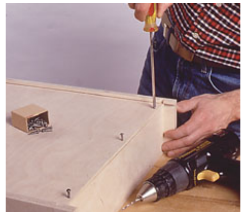
15--Once the bottom is completely seated in drawer, bore pilot holes into the drawer back and install screws. Do not use glue.
