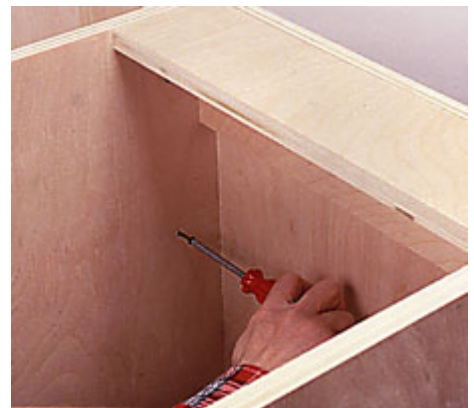
8--Apply glue to the modesty panel, plates and slots and push together. Bore pilot holes and drive screws to tighten the joint.
