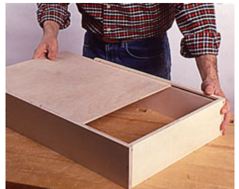
14--Cut the drawer bottom to size and sand smooth with 220-grit paper. Then, slide the bottom into the drawer assembly.
