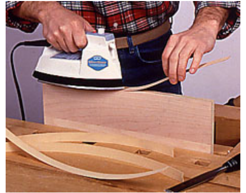
1--Finish the plywood edges with iron-on veneer tape. Set the iron for high heat and press down to activate the hot-melt glue.
