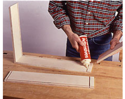
13--Cut the drawer parts to size and finish sand with 220-grit paper. Dust off, then apply glue to all joints and assemble parts.
