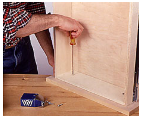
21--Attach the drawer faces to the drawer boxes by driving the screws through the drawer fronts and into the face adjusters.
