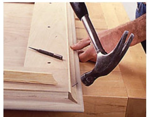
12--After the support strips have been installed on the bottom of the top, miter and nail cove molding to edges of strips.
